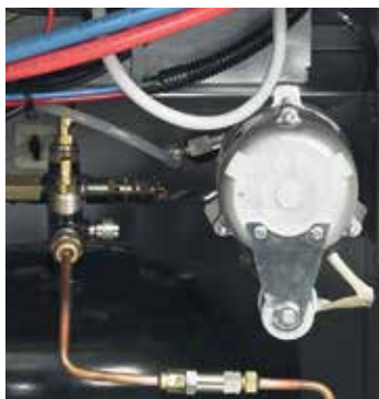
Integrated fluid pump: For charging high-volume A/C systems
